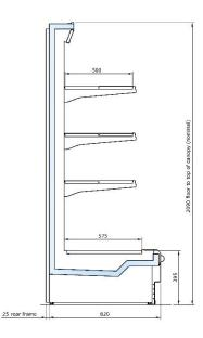
The RJM Crystal is narrow at only 820mm deep with a reduced canopy to maximise product capacity and more importantly, visibility. The structure of the case is specifically designed to suit the heavy load of multiple bottled products and boasts a 400KG/Sq Metre shelf load!
